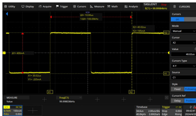
Ideal 400mA 100kHz square wave current measurement
