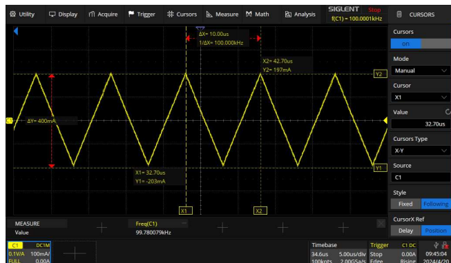
400mA ideal 100kHz triangle wave current measurement
