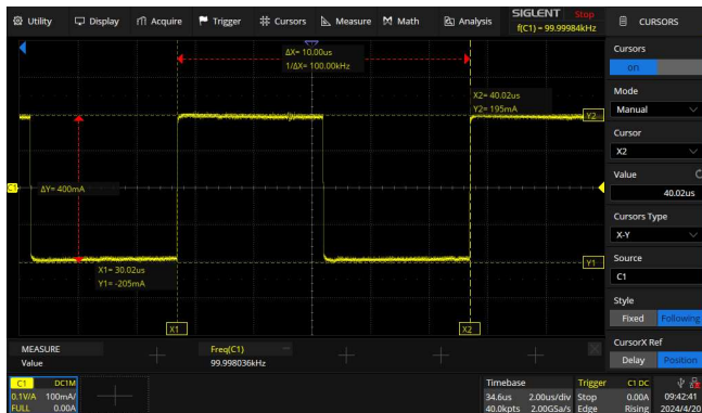
Ideal 400mA 100kHz square wave current measurement
